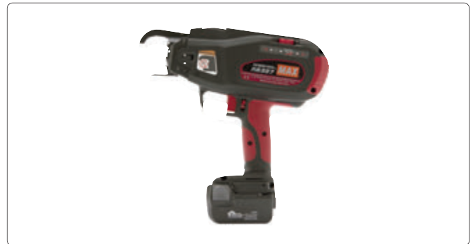
Binding machine The binding machine for fixing the MB System pipes to a reinforcement (e.g. MFF & MTB) is provided for rent against a deposit and fee. Availability should be checked at least 4 weeks prior to site use. 080131 deposit 080301 loan fee up to 2,999 m MB System pipe 080302 loan fee starting from 3,000 m MB System pipe
