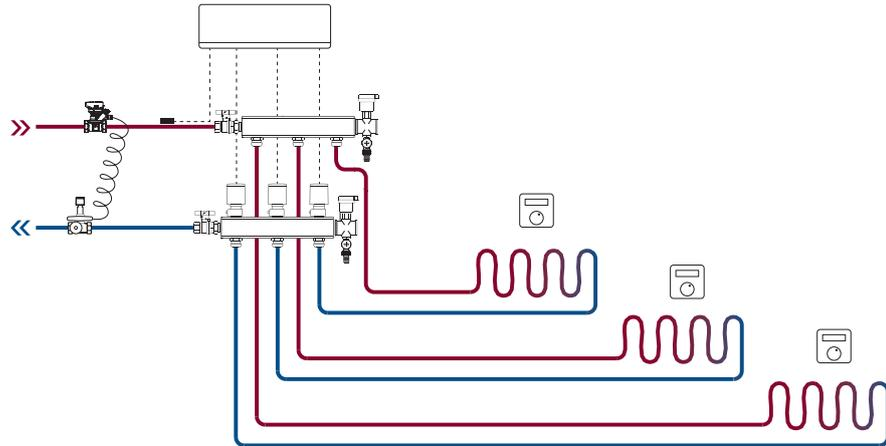
Example 2: 2-pipe system with mixing shunt (optional supply temperature control)
